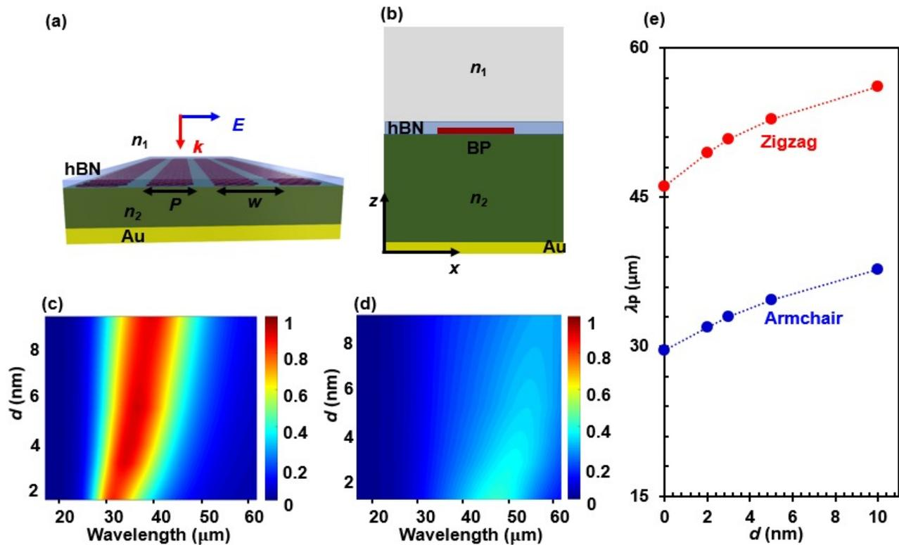
Fig. 4: (a) 3D and (b) 2D schematics of periodic phosphorene nanoribbons enclosed by a hBN layer of thickness  $d$ . The optical response is shown for the (c) armchair and (d) zigzag directions (e) Normal incidence TM mode electric field absorption response for different hBN thicknesses,  $d$  (nm) shown for both armchair and zigzag polarization directions. Here,  $w = 225$  nm,  $n_2 = 1.71$ ,  $n_1 = 1.0$ ,  $N = 2.5 \times 10^{13} \text{cm}^{-2}$ , and  $P = 250$  nm.
