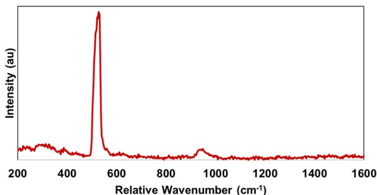
Figure 4. Preliminary data obtained from a Si sample on the custom Raman spectroscopy setup showing the Stokes Raman peak for Si at a relative wavenumber of 528  $\text{cm}^{-1}$ .
