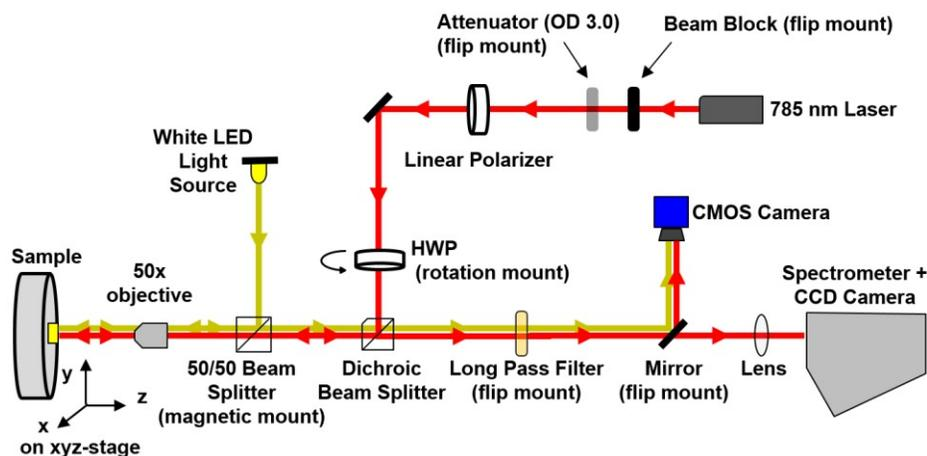
Figure 3. Depiction of the custom Raman spectroscopy setup to be used in SERS experiments with samples created via nanomasking. A 100 mW 785 nm near-infrared continuous-wave unpolarized laser is used for spectroscopy, with a white LED Köhler illumination setup and CMOS camera used for imaging and aligning the sample.
