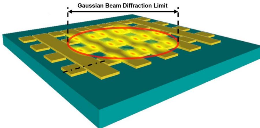
Figure 5. 3D sketch of a grid structure showing illumination over the area of a diffraction-limited Gaussian beam spot causing multiple hotspots due to the presence of nanogaps.
