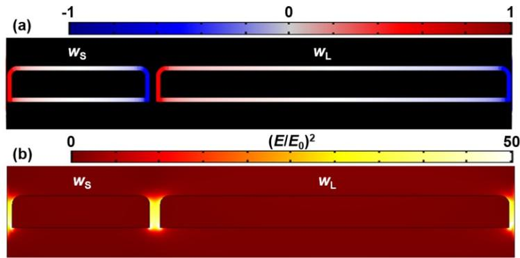
Figure 6. Simulation results of a cross section taken as shown by the cut in Fig. 5 with  $w_L = 165$  nm and  $w_S = 65$  nm as shown in SEM images in Fig. 2. (a) Charge distribution and (b) electric field distribution at 785 nm incident wavelength. Color bars indicate the normalized linear charge distribution and electric field enhancement  $(E/E_0)^2$ . The Si substrate is simulated by using an effective medium,  $n_{\text{eff}} = 1.25$ , surrounding the Au, and so is not shown.
