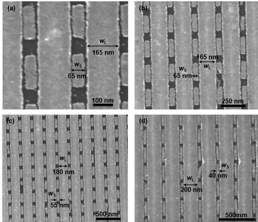
Figure 2. SEM images of dual-width grid structures fabricated using nanomasking with different designed wire widths. The width and spacing of the large wires,  $w_L$ , controls the width of the adjacent wires,  $w_S$ . (a) and (b)  $w_S = 65$  and  $w_L = 165$ . (c)  $w_S = 55$  and  $w_L = 180$ . (d)  $w_S = 40$  and  $w_L = 200$ . All measurements are assumed to have a standard deviation of 3.03 nm.<sup>39</sup>
