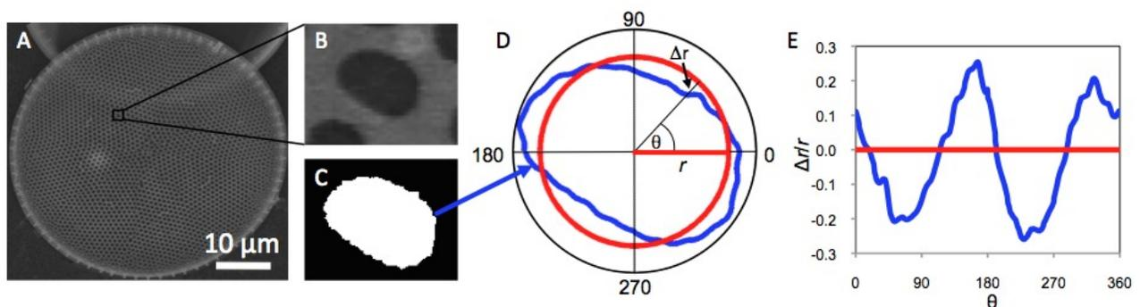
Figure 2. (A) SEM of diatom species *Thalassiosira anguste-lineata*. (B) Single diatom pore. (C) Binary image of single diatom pore. (D) Polar plot of perimeter of diatom pore relative to a circle with an equivalent area. (E) Normalized Cartesian plot of  $\Delta r$  vs.  $\theta$ .
