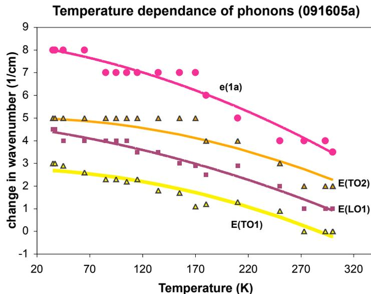
**Figure 6.** The optical phonon energy of sample 091605a as a function of temperature. Each vertical set of data represent a single spectrum mapping to give the phonon frequencies at that specific temperature. The phonon labels correspond to Fig. 4. The lines are the least square fit approximation of each phonon temperature dependence. The least square fit is also an approximation for the phonon energy dependence in bulk GaN.<sup>7</sup>
