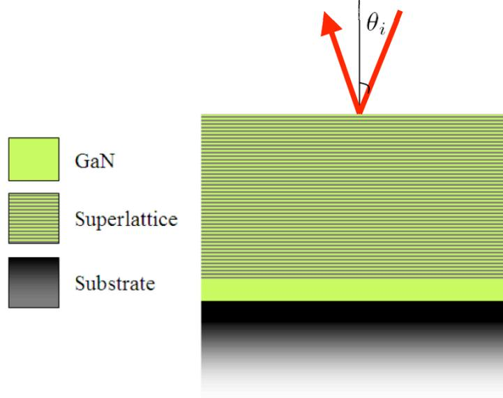
**Figure 1.** Cross section of a sample: superlattice grown on a sapphire substrate. A 30nm GaN buffer is between the superlattice and the substrate. Also illustrated is the reflectivity angle of 15 degrees.
