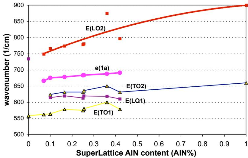
**Figure 4.** Optical phonon energies in each AlGa<sub>N</sub>/Ga<sub>N</sub> sample at room temperature as a function of aluminum concentration. Each vertical set of data represents the phonons present in a single sample. Plotted on the edges are the phonon modes in bulk AlN and GaN. Notice the phonon e(1a) which is a new phonon that exists in the superlattices but not in the bulk.
