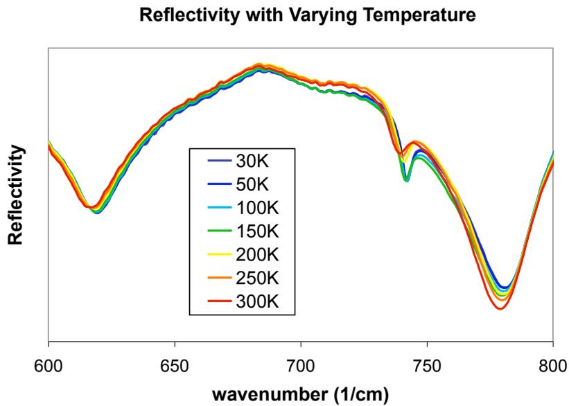
**Figure 5.** The varying reflectivity of sample 092505b as a function of temperature. These spectra are shown in the range from 600-800  $cm^{-1}$  in order for the shift in the minima to be observed. This temperature dependence on the minima of the reflectivity results in a phonon energy dependency on temperature.
