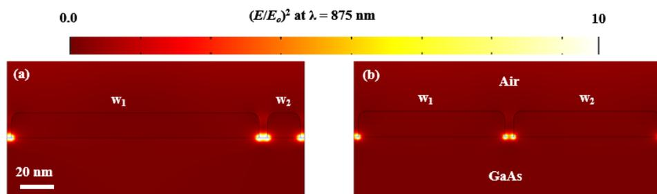
Fig. 1. Optical Enhancement distribution for the same period  $P = 180$  nm, but different wire widths: (a)  $w_1 = 150$  nm,  $w_2 = 20$  nm and (b)  $w_1 = w_2 = 85$  nm. The electric field enhancement in (a) is 19% greater than that in (b) in the GaAs near the gap.
