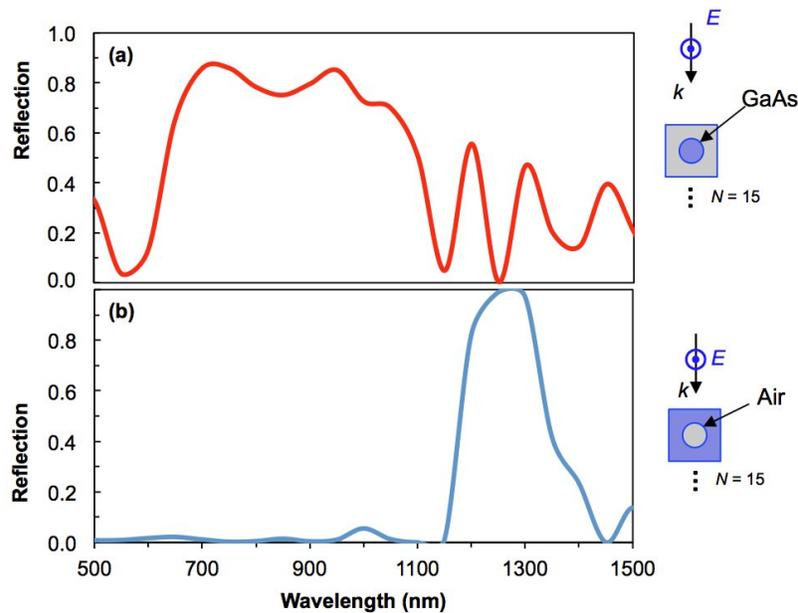
Figure 3. Effects of material properties on PBG. Reflection spectrum for a PC with (a) GaAs posts in air and (b) Air holes in GaAs. Constant parameters are incident light direction, polarization, and  $N = 15$  and  $P = 200$  nm.
