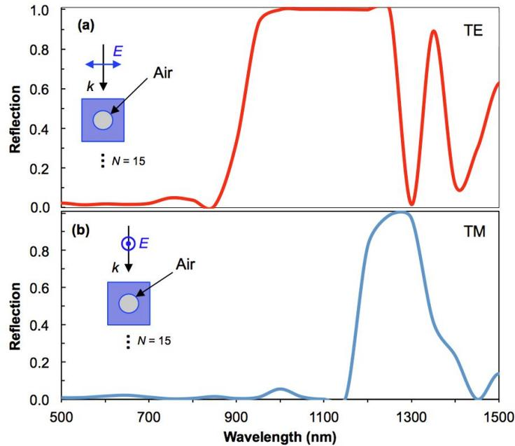
Figure 2. Effects of polarization on the PBG. Reflection spectrum for (a) TE mode and (b) TM mode with  $N = 15$  and  $P = 200$  nm.
