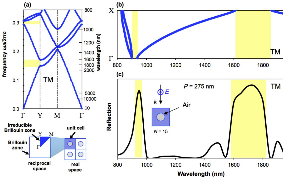
Figure 6. (a) Photonic band structure with unit cell shown in real space and the Brillouin zone and irreducible Brillouin zone shown in reciprocal space. Band structure is for square lattice with air holes in GaAs and with TM polarization. Dielectric constant of 11.8 (b) plots the band structure corresponding to normal incident light parallel to the square lattice as a function of wavelength for the parameters shown: air holes in GaAs, TM polarization,  $P = 275$  nm.
