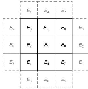
Figure 5. The square lattice shown for a  $3 \times 3$  periodic mesh with the electric field at each position labeled  $E_n$ .
