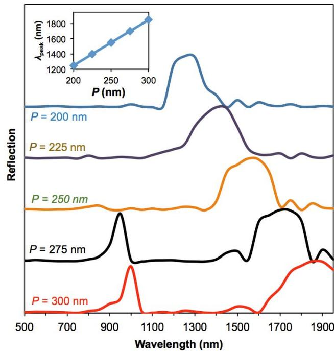
Figure 4. Reflection spectrum for various PCs with different periods ( $P$ ). Constant variable for this figure are  $N = 15$  TM polarization with a PC with air holes surrounded by GaAs.
