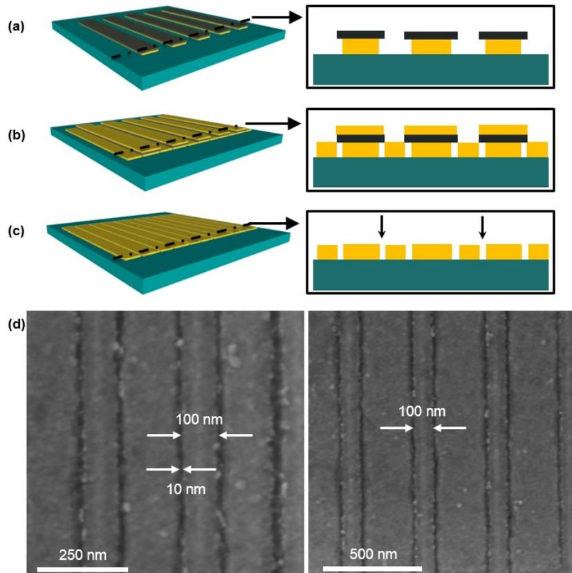
Figure 4. Blanket nanomasking of parallel nanowires. 3D sketches and cross-sectional views of (a) the result after the first lithography process, metal deposition (gold and gray), and Cr layer oxidation (gray), (b) the secondary metal deposition step, and (c) the resulting parallel nanowires separated by nanogaps. (d) SEM images of the resulting Au nanowires.
