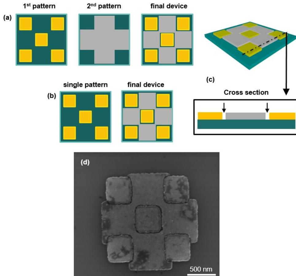
Figure 3. Nanomasking demonstrating the removal of a lithography step. (a) Top views of the first and second lithography patterns and the final result when the two are overlapped. (b) Top views of the first lithography pattern and final device when the second lithography step is removed. (c) 3D sketch and cross sectional view of the final device. (d) SEM image of the result when using the two lithography patterns shown in (a).
