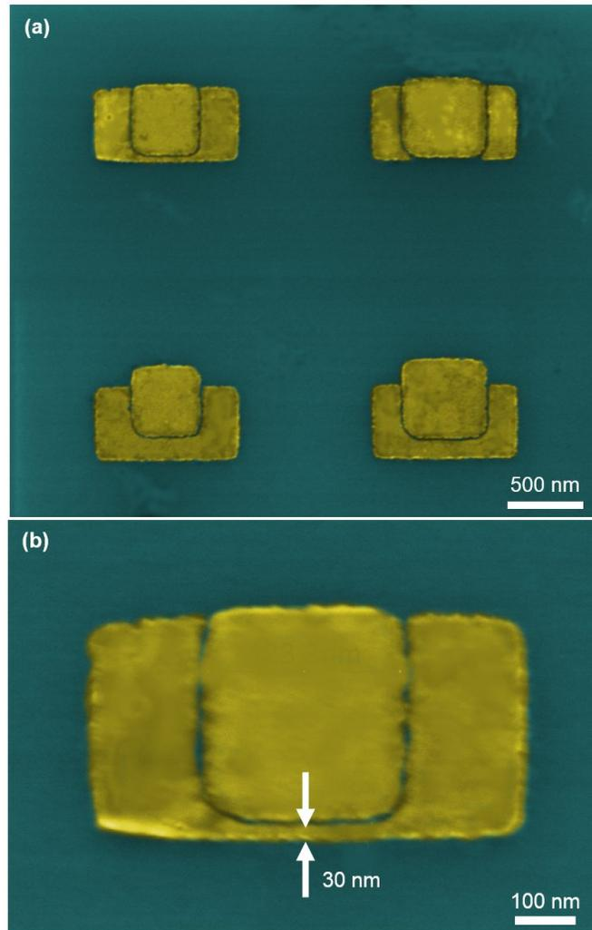
Figure 2. Colorized SEM images of the results of nanomasking fabrication for a square pattern overlapping a rectangular pattern where metal 1 and 2 were both Au. (a) The overlap between the two patterns was changed, as well as the size of the square pattern. (b) Higher magnification image showing the resulting nanostructure width.
