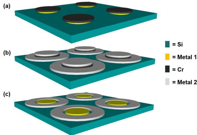
Figure 1. 3D sketch of the nanomasking technique for circular patterns. (a) Metal 1 and Cr shown to have been deposited after lithography step 1.  $\text{Cr}_x\text{O}_y$  overhangs the edge of the metal 1 disks. (b) Metal 2 shown to have been deposited, overlapping the primary structures, after lithography step 2. (c) The result after etching the Cr. Disks of metal 1 separated from rings of metal 2 by a gap.
