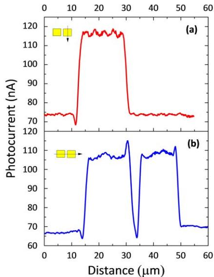
Fig. 4. Photocurrent sweep using red laser across a pair of pads having Au thin-film with thickness of 30 nm for (a) vertical and (b) horizontal scans.
