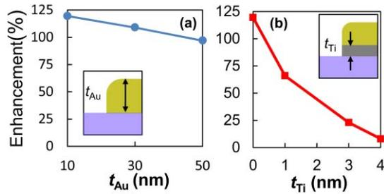
Fig. 3. Enhancement(%) in the photocurrent after applying arrays of: (a) variable Au thickness, and (b) variable Ti thickness.
