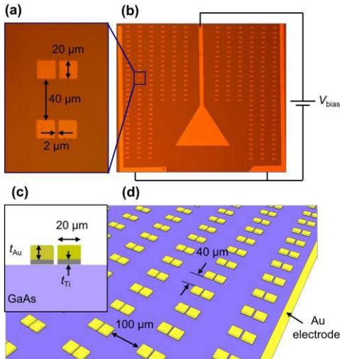
Fig. 1. (a) Microscopic image showing pair of  $20 \times 20 \mu\text{m}$  pads spaced by  $2 \mu\text{m}$ . (b) Top view of the photodetector with the microstructure array. (c) Cross-section view of pads made from thin-films of Au with thickness of  $t_{\text{Au}}$  and Ti with thickness of  $t_{\text{Ti}}$  deposited on GaAs. (d) Schematic showing the microstructure array deposited between the photodetector electrodes.
