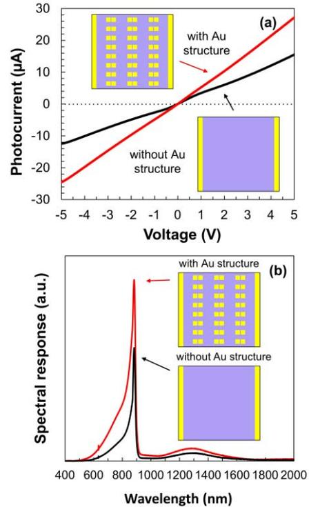
Fig. 2. (a)  $I_{\text{photo}} - V$  curve and (b) spectral response at  $5 \text{ V}$  bias for device before and after applying array of microscale pads with  $t_{\text{Au}} = 50 \text{ nm}$ .
